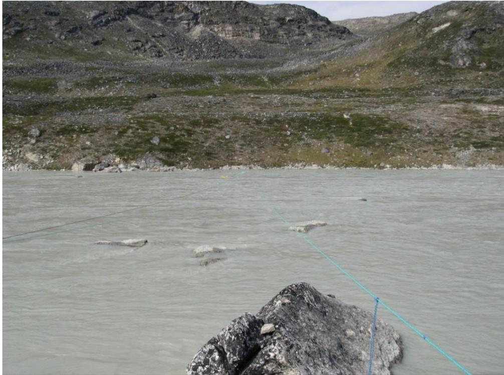
**Figure 8.** Measurement of discharge at the outlet river from catchment 07.d.I. A wire is set up across the river at the measuring cross section and water velocity is measured by an acoustic Doppler current meter (ADCP) mounted on a small yellow catamaran boat, which can be seen near the opposite shore. Photo: Asiaq.
