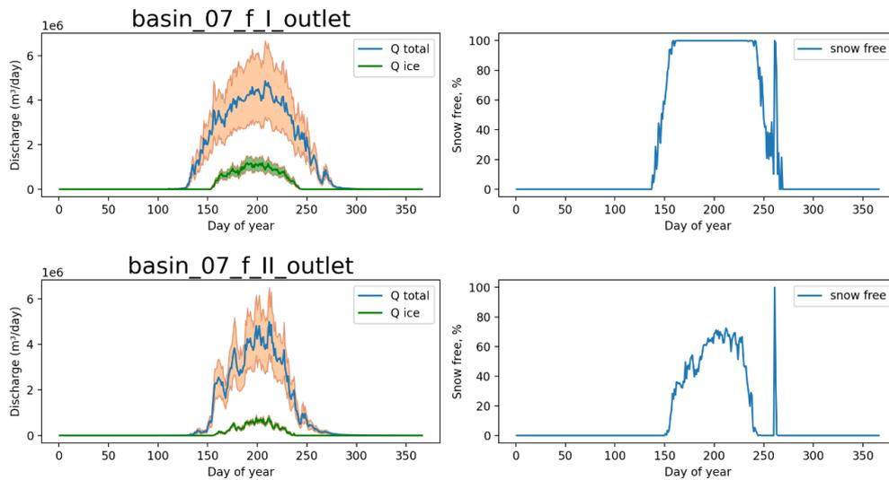
**Figure 68.** Left graphs: seasonal variation of the total daily discharge from the catchment, averaged over 1981-2020 (blue line “Q total”), including uncertainty interval (light brown) with the daily discharge from the glaciated part of the catchment (green curve “Q ice”) specified, also including uncertainty interval (light green). Right graphs: daily percentage of the total catchment (ice-covered and ice-free) experiencing snow-free conditions.
